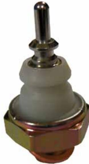
The Thermometrics Oil pressure switch monitors the engine oil flow when the engine starts. It can detect oil pressure and enables the EMS ECU to check for the lack of oil. It can also send an alarm signal to the driver, helping to avoid engine damage due to overheating.
