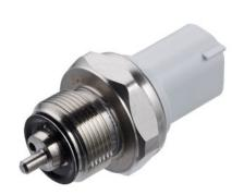
The CCT high-pressure temperature sensor was specially developed for the high pressures and temperatures in CO2 heat pumps (R744). Such heat pumps are primarily used in thermal management in vehicles with electric drive (EV). Thanks to its robust stainless steel design, the sensor withstands the high pressures and temperatures in this application.
